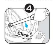
HOLD ON THE CENTRE OF HANDLE TO OPERATE THE TORQUE WRENCH. STOP WHEN YOU HEAR A 'CLICK'. THIS MEANS YOUR TORQUE MEASUREMENT HAS BEEN REACHED
